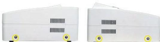
Fig. 7-3 Instrument case fixing screws
