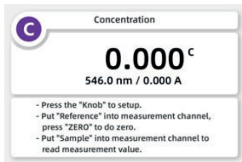
Fig. 6-5 The calibration standard sample measures the unknown sample concentration
