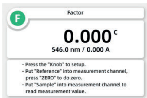
Fig. 6-9 Enter the equation coefficient to measure the concentration
