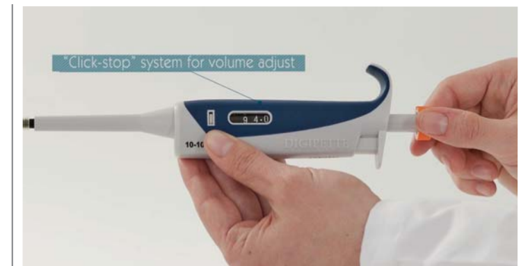
“Clik-stop” mechanism of volumen selection
