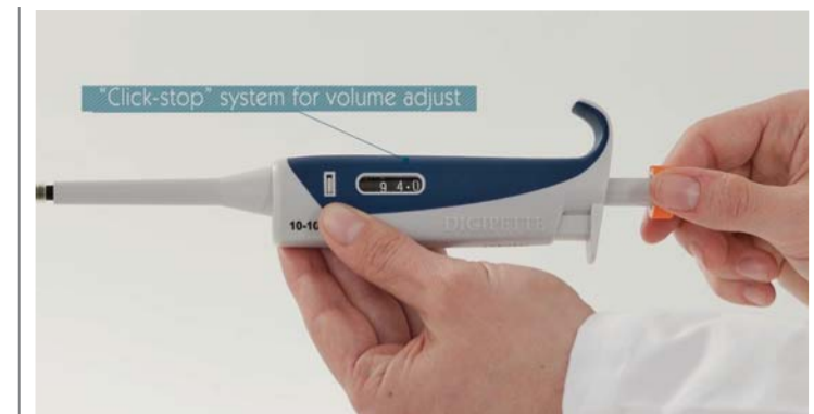
“Clik-stop” mechanism of volumen selection
