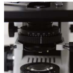
[5] Mechanism of centring the condenser
